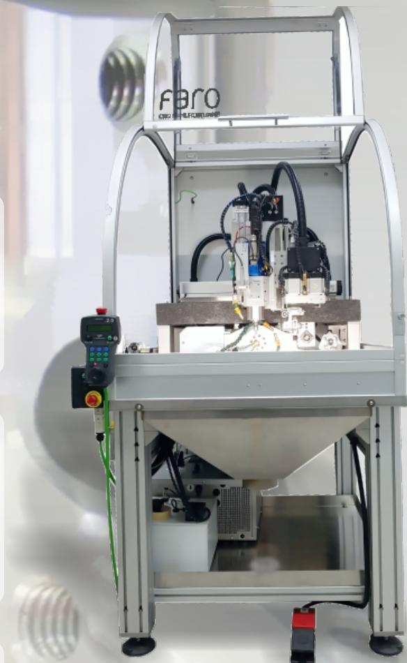
F35 is the most versatile and popular 5-axis equipment in the compact class of CNC machine tools for all accurate engraving, diamond-cutting, drilling and stone pre-setting tasks on different materials of beads, half round and flat rings, wedding bands and hollow bangles, even oval and of irregular shape.
